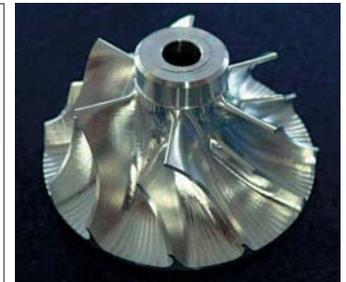
A machining Example (impeller for automobiles)
