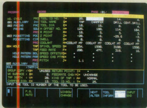
切削条件自動決定画面 Cutting data screen (On which are automatically determined)
