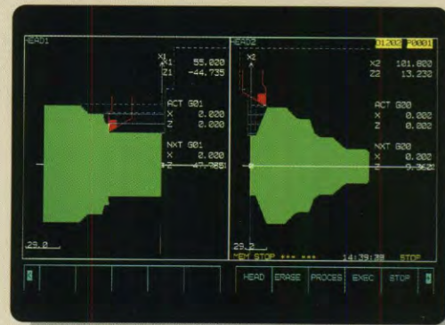
2系統旋盤のアニメ描画面 Animated simulation screen of a 2-path lathe
