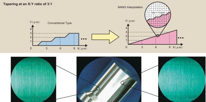
**Conventional interpolation** Streaks may be made on the machined surface due to the computation error produced by the units used for commands.
