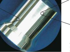
NANO Interpolation A streak-free high-quality machined surface can be made by precision computation in nanometers.
