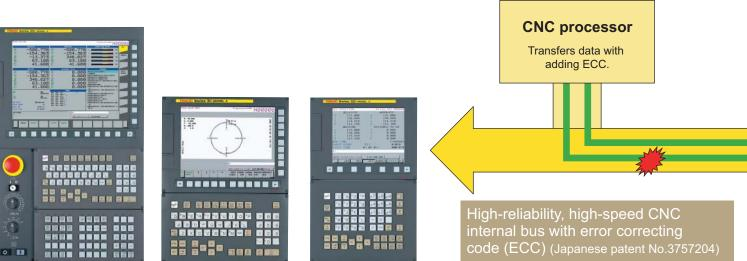
15-inch color LCD unit, QWERTY keyboard, standard machine operator's panel
